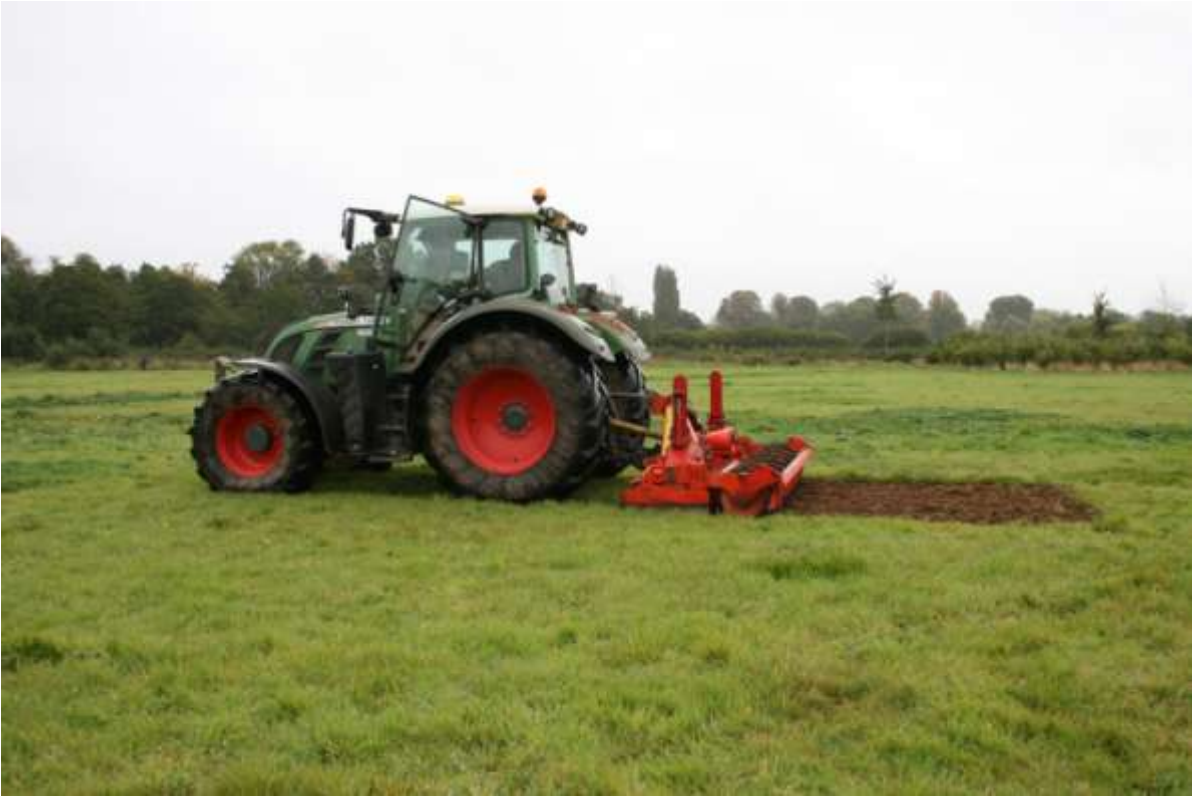
Figure 5: Testing the depth of the power harrow and roller. This was following a relatively dry period of weather with a single brief shower just prior to the works (photograph taken on 3 rd September 2015).
