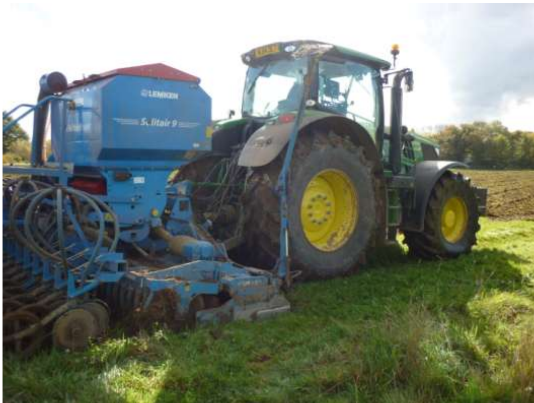
Figure 7: tractor with power harrow, seed hopper and roller (photograph taken on 28 th October 2015)
